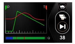
Once the desired profiles have been set, it is possible to verify during brewing that the actual temperature and pressure are following the chosen profiles and that the quantity dose is correct. All checks are carried out in real time without waiting end of brewing. Coffee extraction becomes a real-time dialogue between barista and machine, with the aim of increasing man-machine interaction to achieve the best product in the cup.
